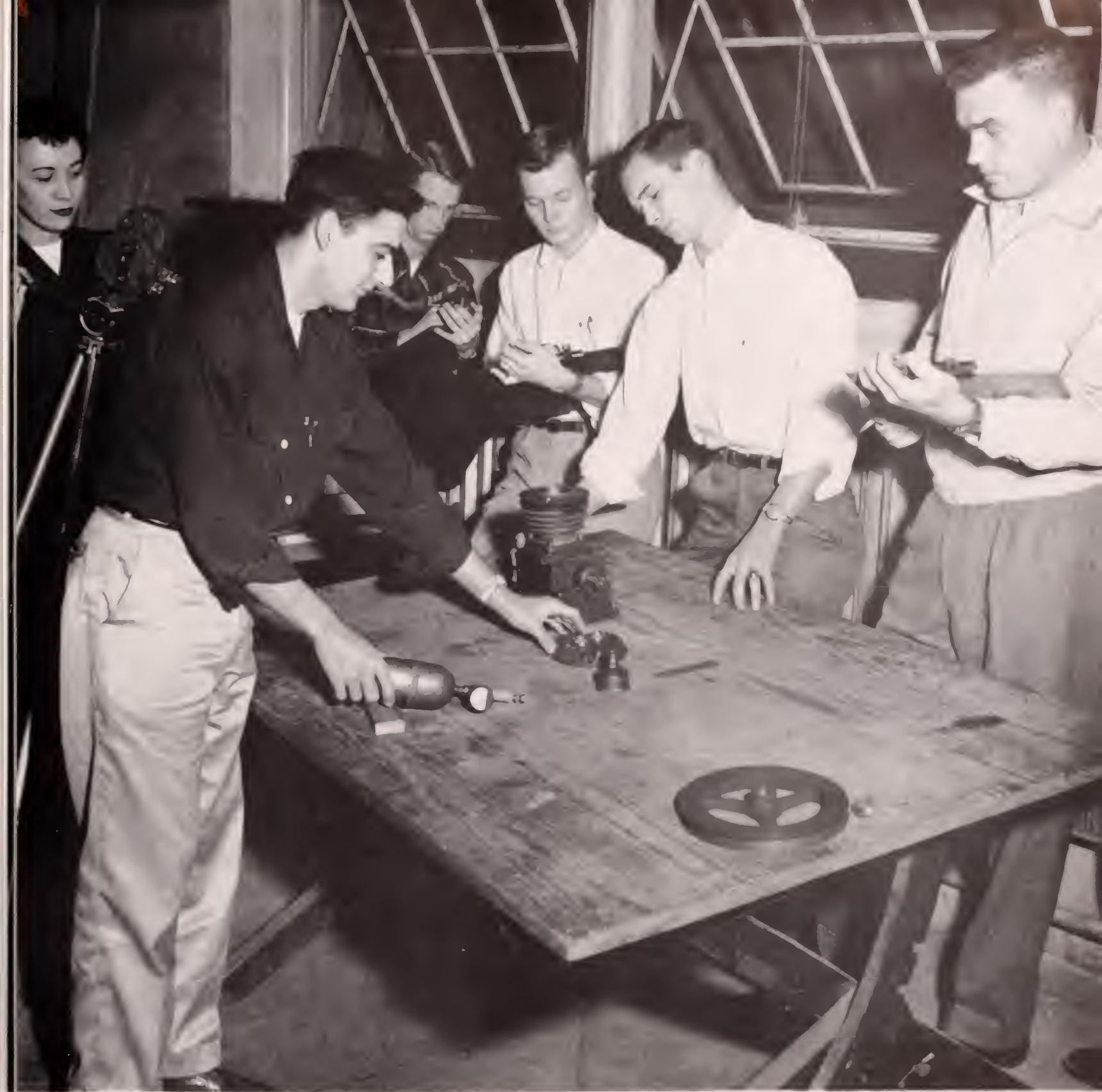
Richard Monsour and George Shackelford are being timed by fellow students as they take apart a compressor. Their movements are filmed so as to catch wasted movement.
